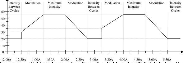
If two or more light cycles overlap, the active light cycle will finish before the new one activates. This situation may be caused by unusual programming or by a period change.
